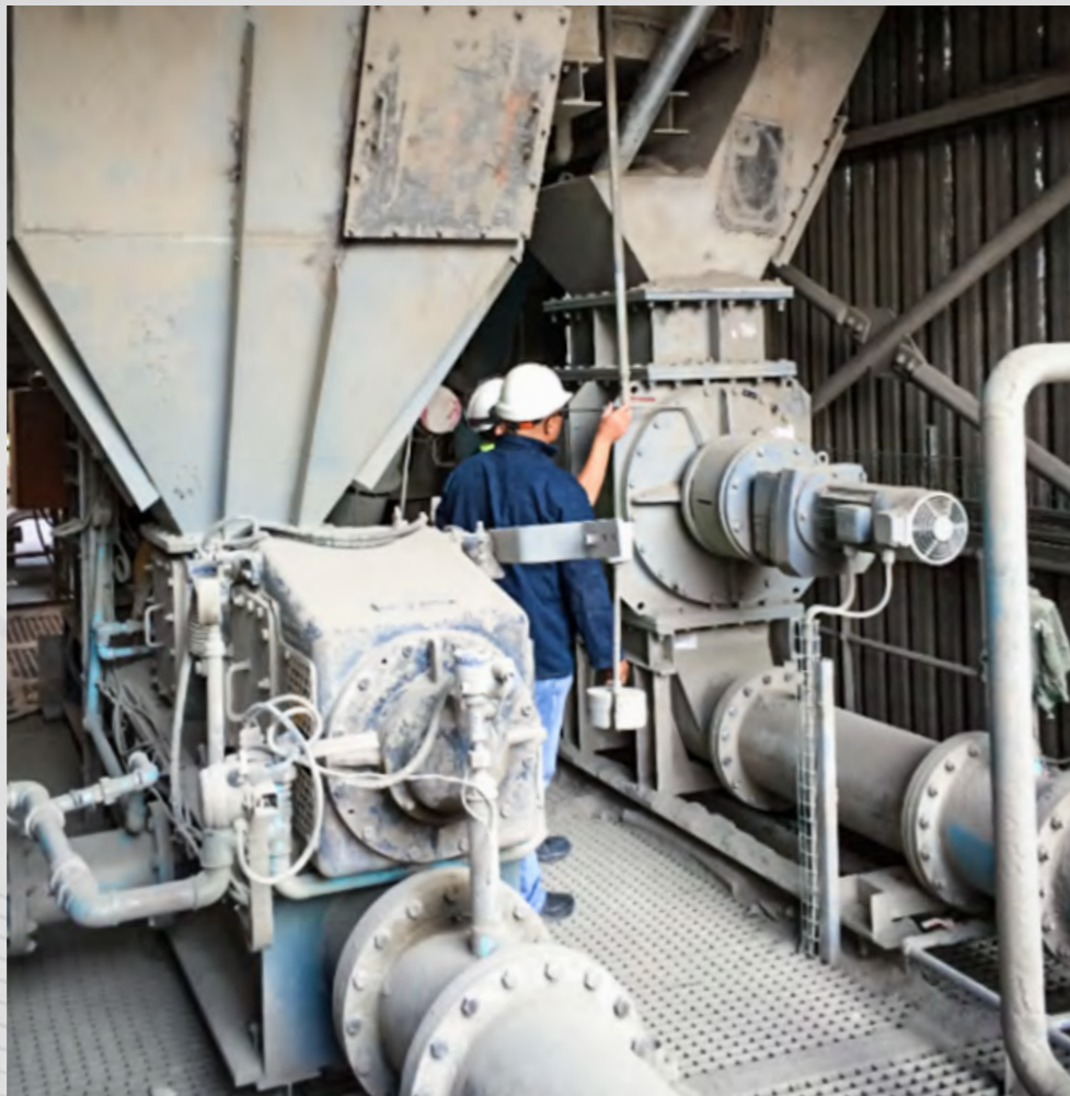
Exchange of Screw pump against KREISEL ceramic rotary feeder
