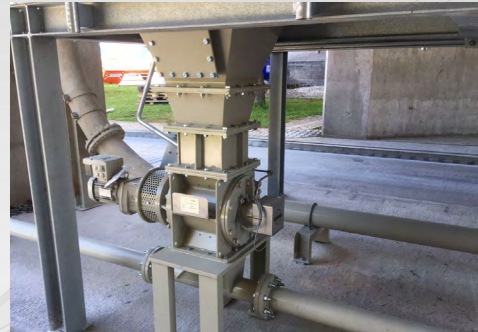
Typical installation of a KREISEL-ceramic rotary feeder
