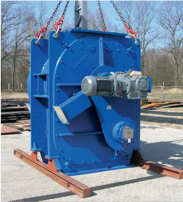
Figure 3: The new rotary feeder with scraper, ready for despatch to the cement works
